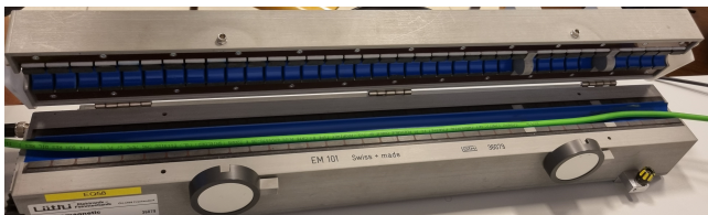
Fig. 12. Disturbance injection clamp conform to IEC61000-4-6
